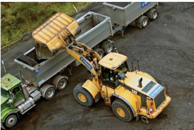
Plate 2 – Loading of ROM Coal into a B-Double Truck at the Tasman Underground Mine
