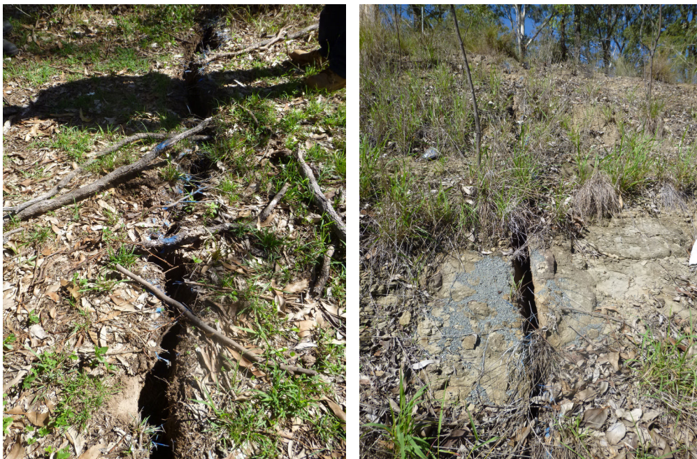
Figure 3.12 Photographs of Typical Surface Cracking in SMP Area 3 at the Abel Underground Mine (110 metres to 140 metres Depth of Cover)
