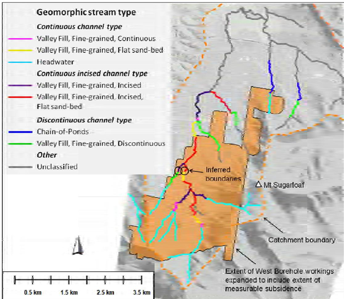
Figure 10. Stream network of the study area classified by geomorphic type. At two locations within the proposed West Borehole Seam workings Project area the stream type boundaries were inferred, because access to the channel was unavailable in the area.
