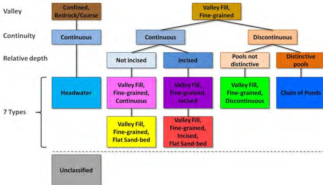
Figure 3. The seven geomorphic stream types (plus Unclassified type) identified in the Surveyors Creek catchment study area.
