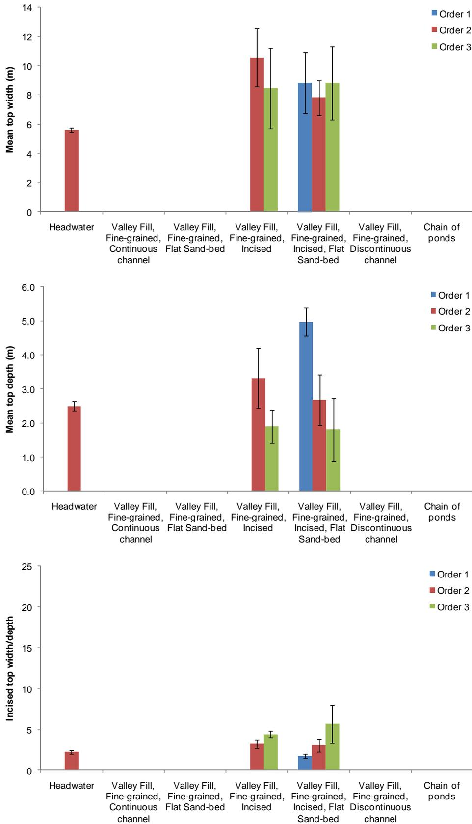
**Figure 15. All classified streams in Surveyors Creek 1 and 2 catchments (plus a small area of upper Wallis Creek catchment). Mean (and standard deviation) of incised channel dimensions, grouped by stream order and geomorphic type.**
