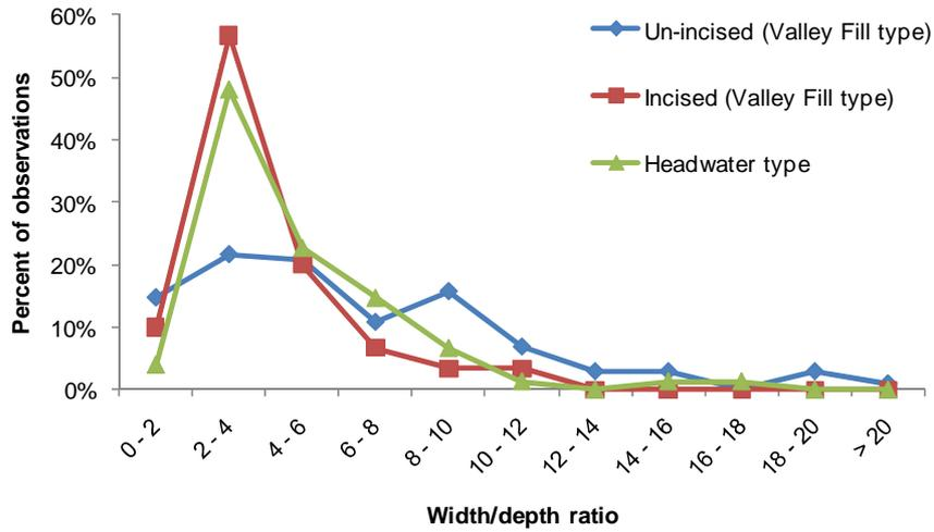
Figure 18. Distribution of width/depth ratios observed for incised and un-incised channel forms of Valley fill stream types and Headwater stream type in the proposed West Borehole Seam Project area.
