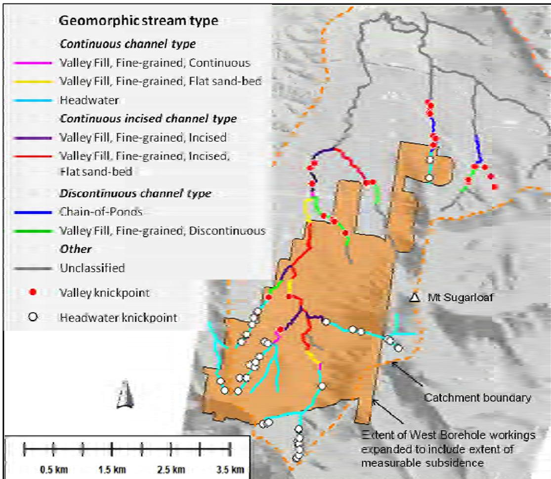
Figure 19. Knickpoints observed in the channel network of the Project area relative to Stream order.
