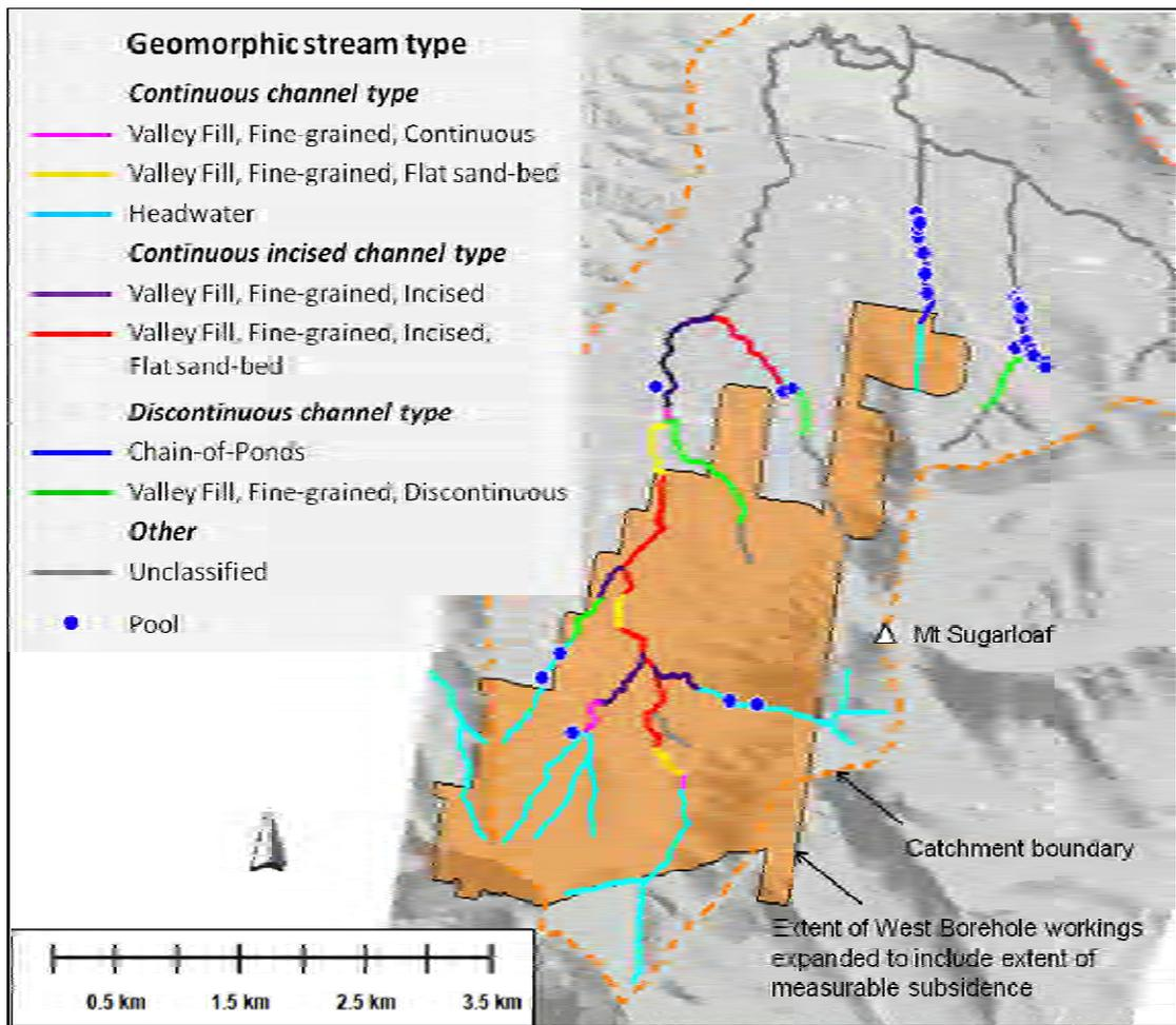
Figure 26. Significant pools observed in the channel network of the Project area relative to geomorphic type.
