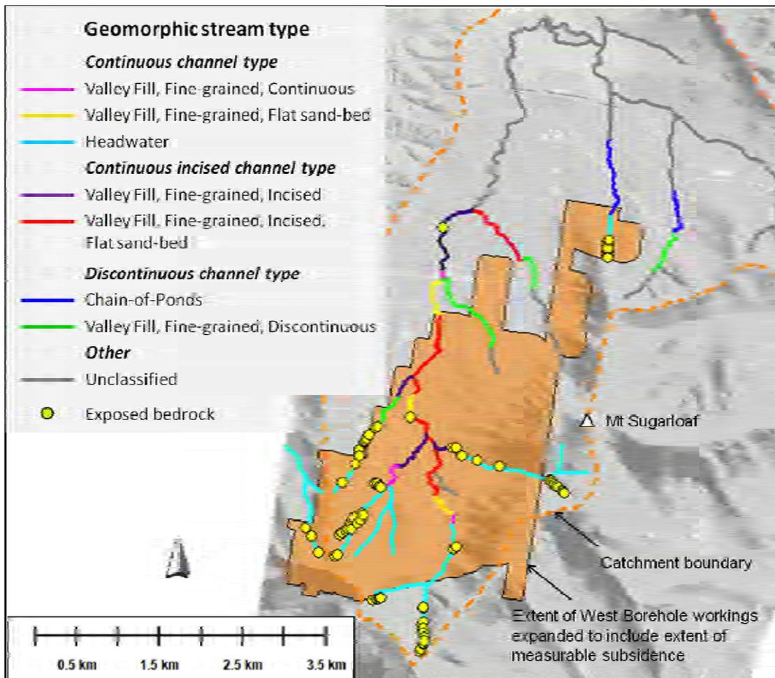
Figure 31. Bedrock outcrops observed in the bed of channel network of the Project area, relative to geomorphic type.
