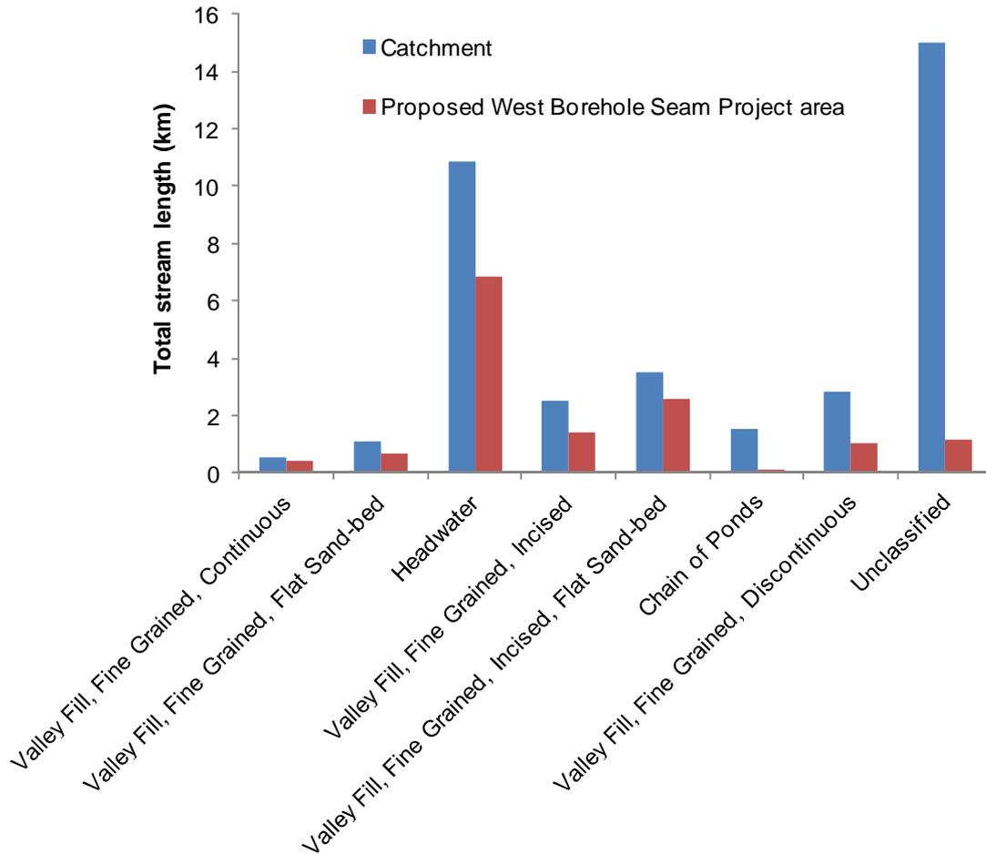
**Figure 11. Total length of streams classified by stream geomorphic type, for the Surveyors Creek 1 and 2 catchments (plus a small area of upper Wallis Creek catchment), and the area within the proposed West Borehole Seam Workings.**
