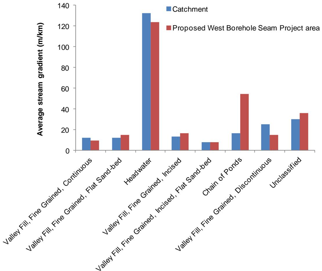
Figure 13. Mean gradients of streams, classified by stream geomorphic type, for the Surveyors Creek 1 and 2 catchments (plus a small area of upper Wallis Creek catchment), and the area within the proposed West Borehole Seam Workings.
