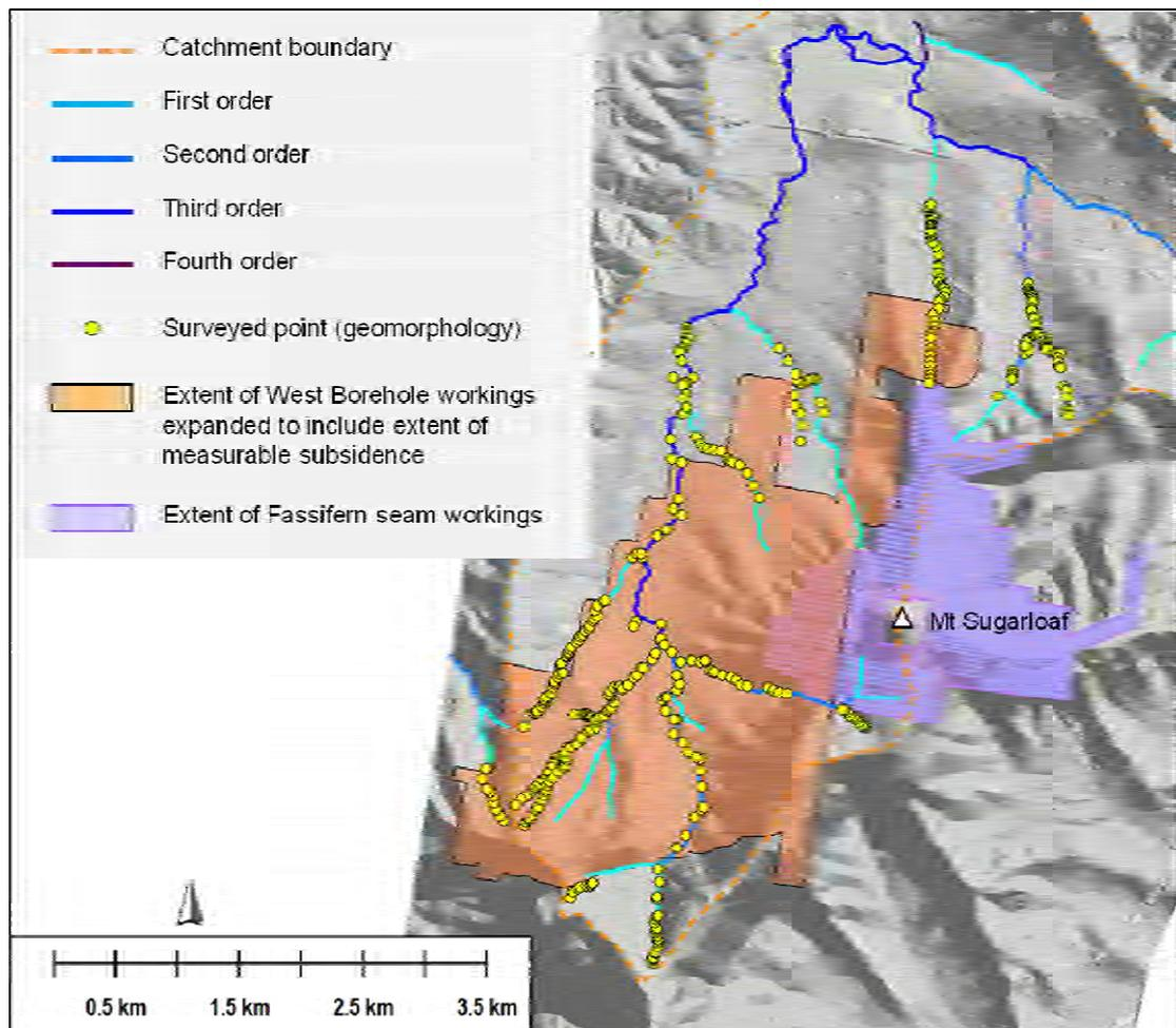
Figure 1. Streams (blue lines on 1:25,000 topographic sheet) within Surveyors Creek catchment in the study area classified by Strahler stream order. Locations of the 385 points included in the fluvial geomorphology field survey are indicated. Also shown is the extent of the proposed West Borehole Seam workings, expanded to include the extent of measurable subsidence (if outside boundary of mine workings). The extent of current and past workings in the shallower Fassifern seam is also indicated.
