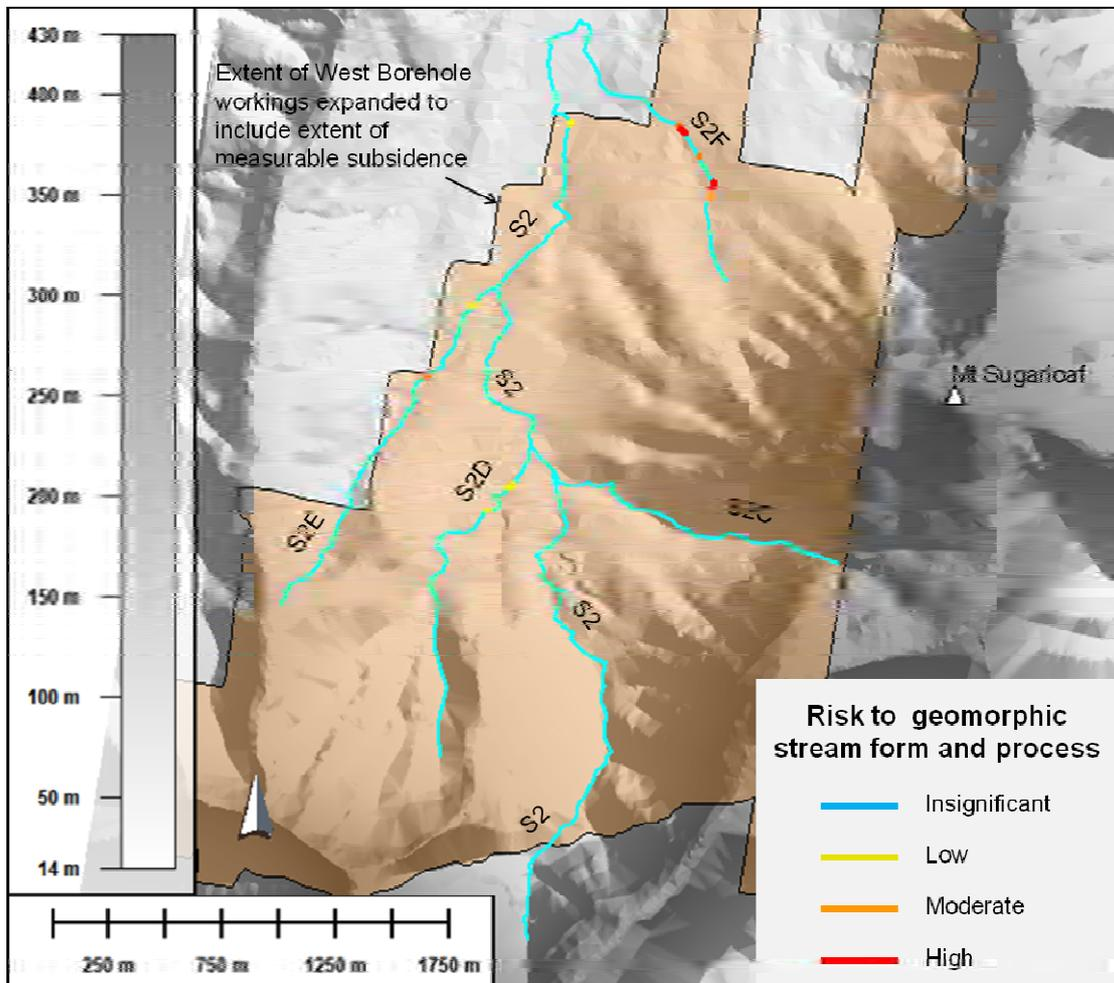
Figure 36. Assessed risk to geomorphic stream form and process under the condition of predicted subsidence with SCZs. Only the streams with subsidence predictions are shown.
