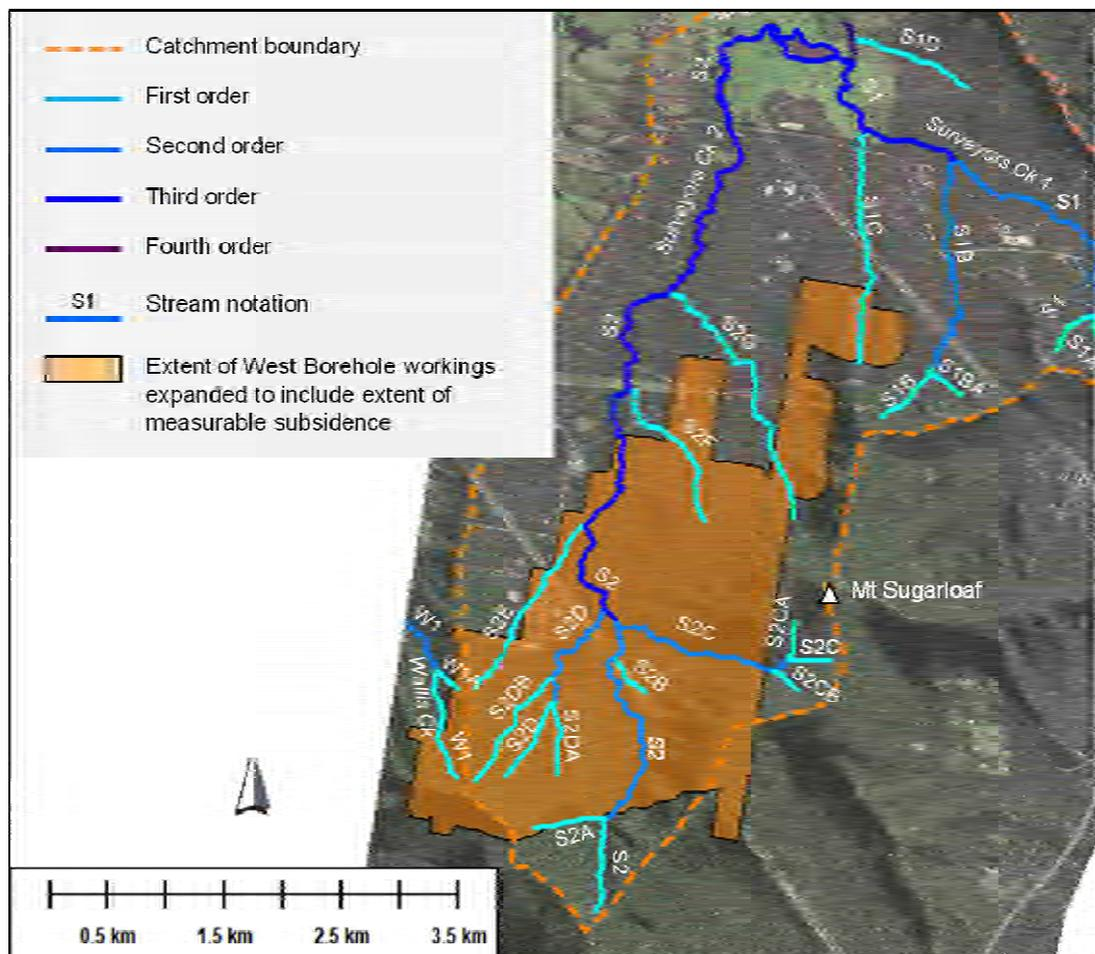
Figure 2. The naming convention used in this report for streams in the study area. Streams classified by Strahler stream order.
