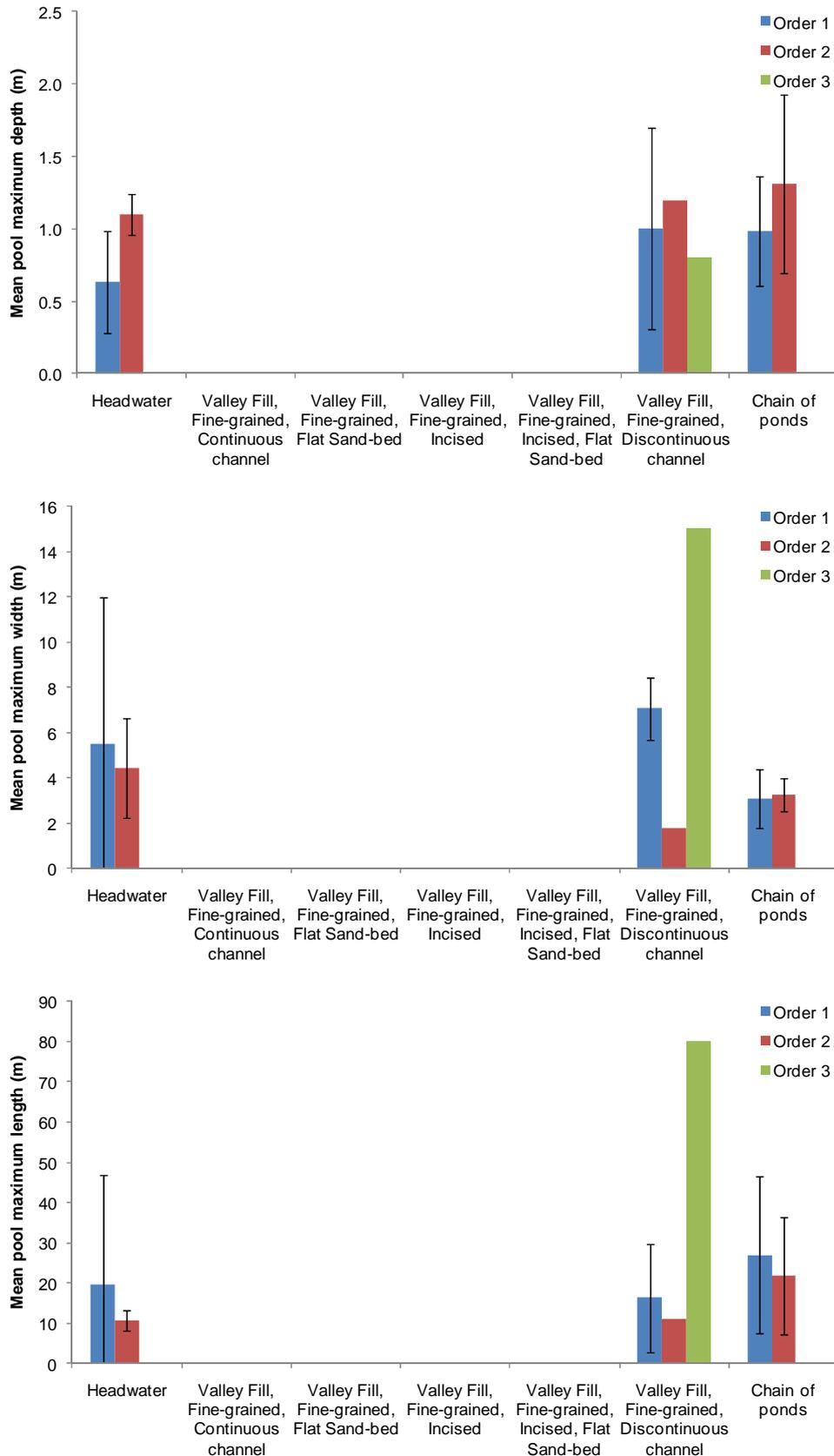
**Figure 27.** All classified streams in Surveyors Creek 1 and 2 catchments (plus a small area of upper Wallis Creek catchment). Mean (and standard deviation) of maximum depth, width and length of pools, grouped by stream order and geomorphic type. No standard deviation indicates 1 or 2 cases only.
