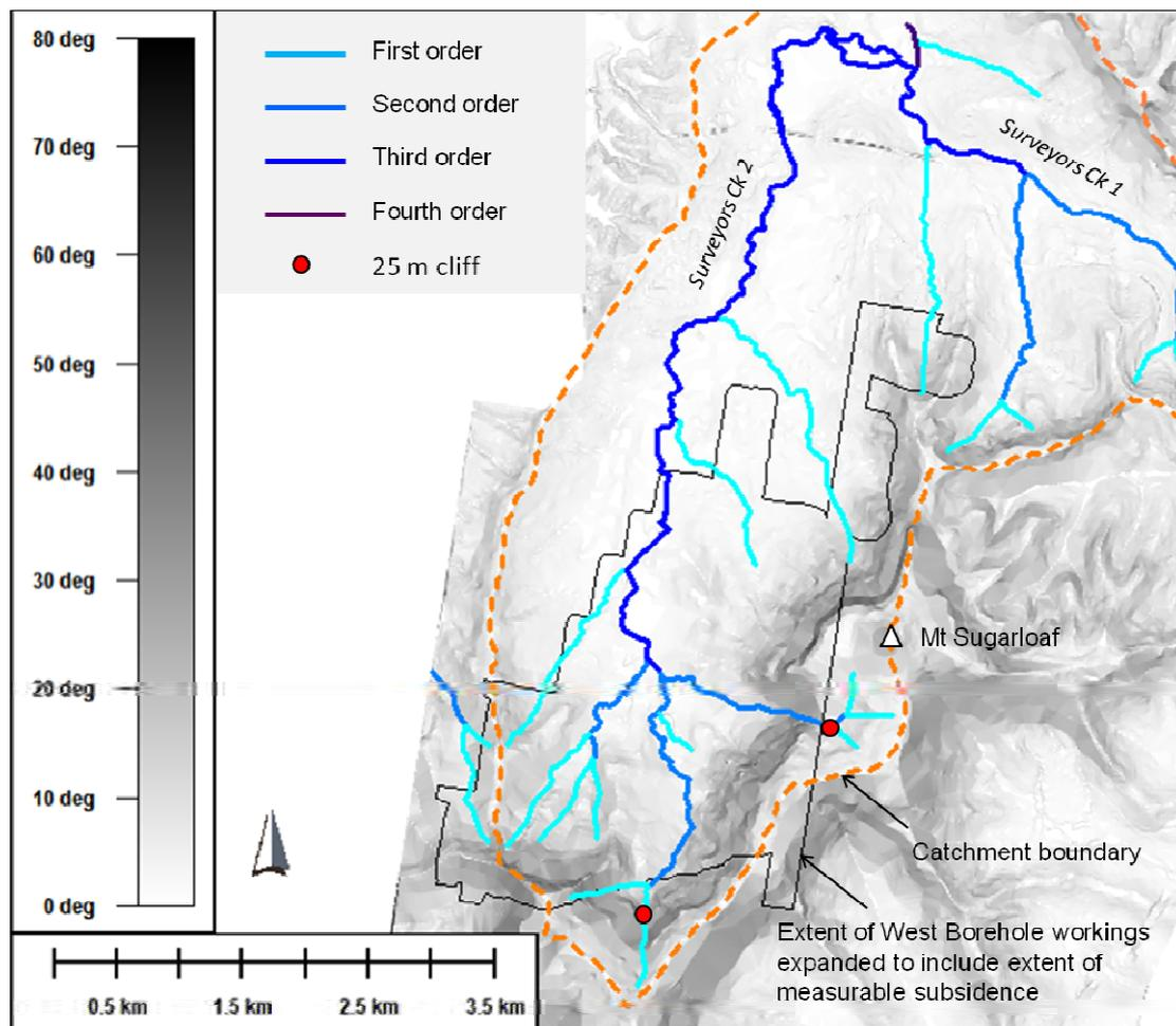
Figure 6. Topography of the study area showing the stream network in relation to slope in degrees.
