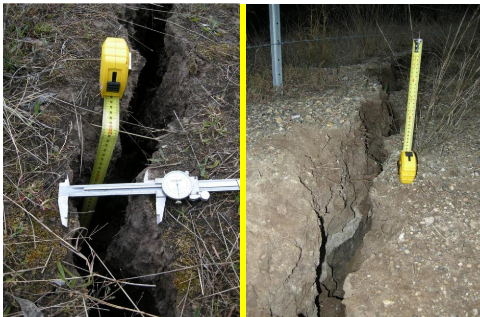
Plate 5 Typical Surface Cracking in the Hunter Coalfield (Less than 100 metres Depth of Cover)
